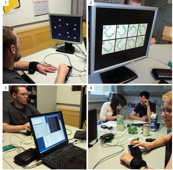
Figure 7: Picture 1 shows the experimental arrangement from a test person’s view sitting about 1m in front of the screen. The elastic wrist support is mounted on the left forearm and the right hand is used to push a button (response on the primary, visual task). Picture 2 shows the screen presented after each trial and requesting a spoken feedback of the recognized tactile sequence (one out of A–H). Photo 3 shows both software and hardware environment as used in the studies, photo 4 finally shows interactions taking place in the distraction zone while conducting an experiment.
