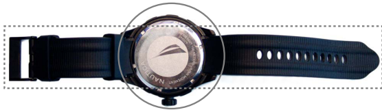
Figure 2: The design space for wrist watch tactor placement: (i) “face”, underneath the watch face, (ii) “wrist”, along the band (upper part).
