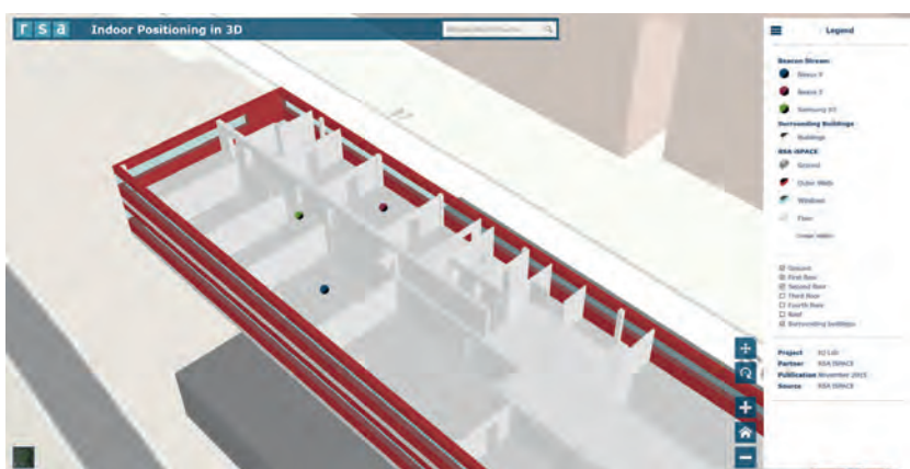
▲ Figure 3: The prototype with the building as a fully interactive model in a web app. The user's position in 3D can be shown as a point in the building.
