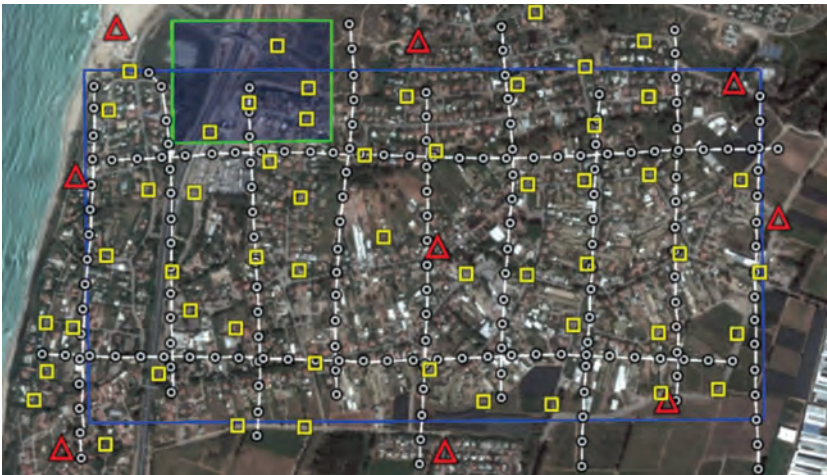
▲ Figure 2: Test site with control points and flight lines.
