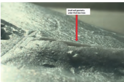
▲ Figure 4: Detail of the small wall in the resin-based 3D model.
