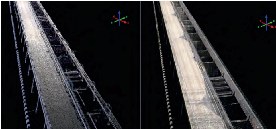
▲ Figure 3: Photogrammetric point cloud after cleaning (left) and Lidar point cloud; point clouds coloured by RGB value.
