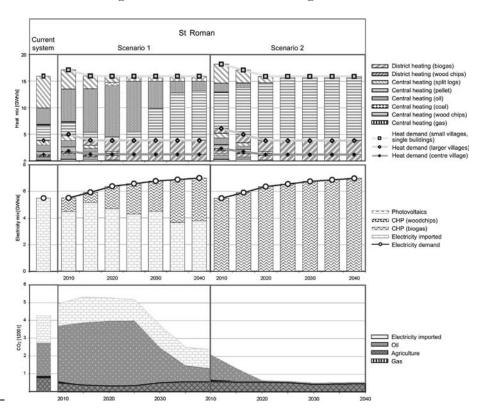
**Figure 8.** Heat mix, electricity mix, and CO<sub>2</sub> emissions for Scenarios 1 and 2 in the St Roman test region
