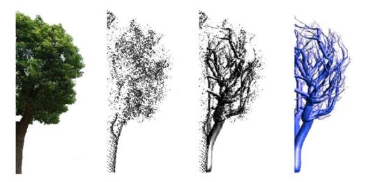
Figure 1. Bottom-up approach to 3D object extraction from a LiDAR point cloud.
