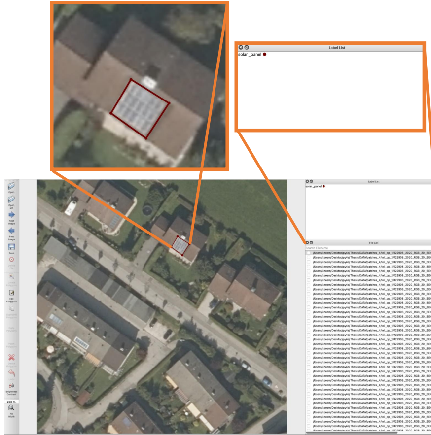
Figure 6.2: Data annotation using labelme tool.
